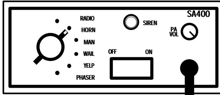
The **OFF/ON** Rocker Power Switch controls the siren power. The siren may be left on any time the vehicle is in operation. The power should be turned off when vehicle is not being used to conserve battery power.
